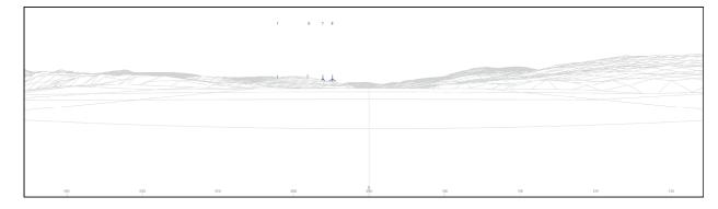
Millenderdale Wind Farm Viewpoint Information Grid Reference 213146E 590040N Ground Height 244m AOD Angle of View 90° Viewing Distance450mm Viewing Distance450mm Layout Information Hub Height 75m Height to Blade Tip 125m Nearest Visible Turbine 4728m Number of Sets of Tips visible <sup>1</sup> 4 Number of Hubs visible <sup>1</sup> 2 Turbine visibility <sup>2</sup>078° to 089°
